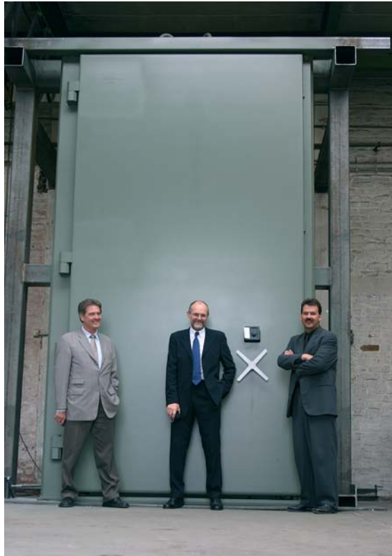
The 4.40 high strongroom door, during final assembly at the manufacturer's works before shipment
