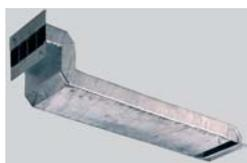
Ventilation shaft for overhead ventilation, zinc-coated; Dimensions: 130 (190) mm x 210 mm x 855 mm (hwxwd); Cross-section of ventilation area: approx. 100 cm<sup>2</sup>
