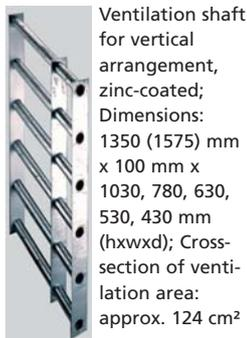
Ventilation shaft for vertical arrangement, zinc-coated; Dimensions: 1350 (1575) mm x 100 mm x 1030, 780, 630, 530, 430 mm (hwxwd); Cross-section of ventilation area: approx. 124 cm<sup>2</sup>
